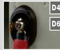
1-point closure with disconnectable lock-holder hasp (shackle with 6 to 7 mm Ø recommended)
